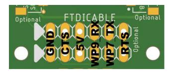
The pinout of the FTDI connector is shown above. The CTS and RTS lines are not used by the Serial Wombat 18AB PCB board. The dual row of headers is designed to make these lines accessible should the user want I/O lines that are controlled directly by the host rather than the Serial Wombat 18AB chip.
