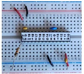
I2C lines should be pulled up with appropriate resistors. Appropriate values vary with application and clock speed. 2200 ohm pull up resistors are suggested as a starting point. Reliance on internal Arduino or other micros' pull ups instead of discrete resistors may cause communication errors.
