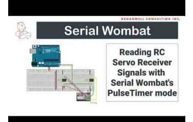
Here's an Arduino example of the Pulse Timer pin mode from the Arduino library examples which reads the high time of 4 channels of an R/C servo receiver:
