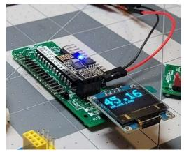
ESP-01 modules with their onboard ESP8266 WiFi enabled SOC provide an exceptional value in terms of wireless connectivity and processing power for the price. However, they are lacking with regard to I/O capability. When combined with a Serial Wombat 18AB chip, the ESP-01 becomes a very reasonably priced IOT powerhouse.
