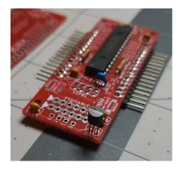
The Serial Wombat 18AB chip power supply should never exceed 3.6V (3.3V recommended). Therefore, it cannot be directly powered by a 5V supply. For convenience, the Serial Wombat 18AB PCB board incorporates options for adding a 3.3v regulator (not included). Mounting locations are available for either a TO-92 through hole part and input and output capacitors (C5V and C3V3, 0.1" pin spacing) or a SOT23-3 surface mount part and 0603 sized input (C4) and output (C5) capacitors.
