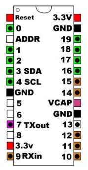
Shown above is the pinout of the Serial Wombat 18AB chip. Pins marked in Green are capable of Analog input functions in addition to digital functions. Pins marked in brown can tolerate 5 volt digital inputs (input voltage to other pins should not exceed the chip supply voltage, typically 3.3V). Pins with circles are capable of enhanced digital performance pin modes.
