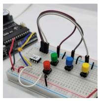
Debounced Input pin mode is designed to facilitate button and other switch style inputs which may oscillate before settling to a constant value.
