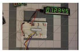
Driving a TM1637 sevensegment display using the Serial Wombat 18AB chip
