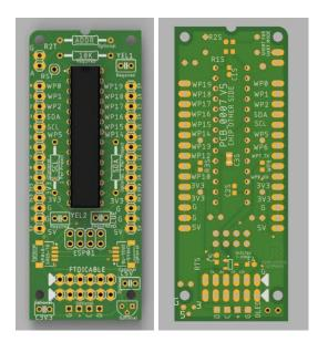
The Serial Wombat 18AB PCB Board is designed to make the Serial Wombat 18AB chip convenient to use alongside other hobby electronics boards. It is designed to support a number of different use cases, including I2C connection, UART connection through an FTDI or similar USB to UART cable and standalone IOT board when combined with an ESP-01 ESP8266 module.
